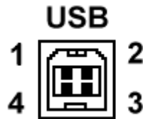
Figure 3-3: USB Connector pin orientation.
